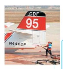
ex-Navy planes that line up to refill 1,200 gallons of flame retardant at a time — a process that takes about four minutes for
